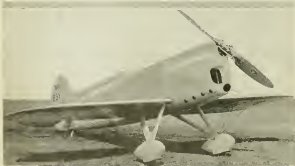
The Brown Special, powered with the 4-cylinder 185-h.p. Menasco C-4-S Pirate engine
